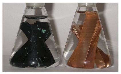
**Above:** Appearance of copper after 15 years of exposure in distilled water at room temperature. Hydrogen from corrosion can escape from the left container but not from the container to the right. The water volume was equal in the flasks in beginning of the exposure.
